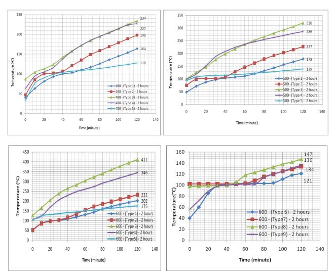
Figure 6: Temperature measured under coatings exposed to 600°C for 2 hours.
