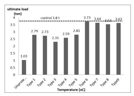
Figure 11: Failure loads for protected FRP-strengthened RC beams exposed to 600°C.
