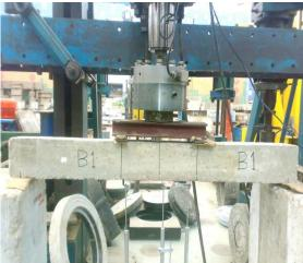
Figure 4: Compression machine for testing cubes and 4-point bending test for beams
