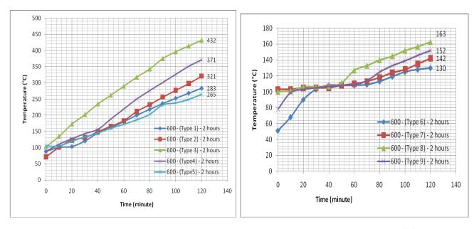
Figure 9: Temperature measured under coating types 1-5 when exposed to 600°C for 2 hours.
