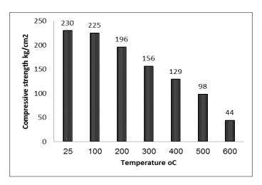
Figure 5: Compressive strength of unprotected cubes after exposure to elevated temperatures.
