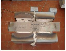
Figure 3: Installation of concrete cubes and beams in the electric furnace.
