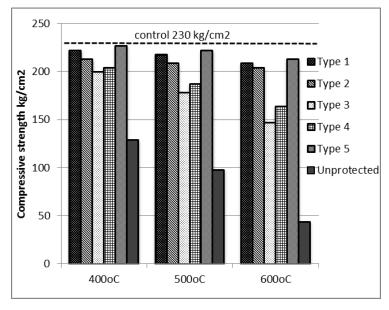
Figure 7: Compressive strength for protected cubes with coating types 1-5 when exposed to 400,500 and  $600^{\circ}$ C 2 hours.
