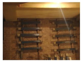
Figure 2: RC beams strengthened by FRP
