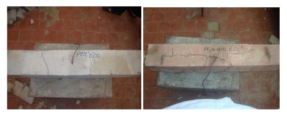
Figure 10: FRP-strengthened RC beams protected using type 1 and 4 after exposure to 600°C.
